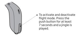
Opening and closing the battery drawer will deactivate the flight mode. See section: Quick reset.
