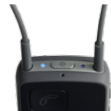
Bring Streamer Pro into pairing mode by pressing the on/off button on the top of Streamer Pro for approximately 5 seconds until the blue light starts blinking.
