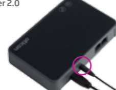
...and the mini jack connector to the Phone Adapter 2.0's AUX in/out port.
