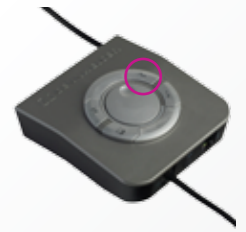
Ensure the headset/handset button on the UI770 box is deselected (not pressed down).
