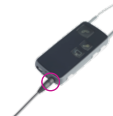
Connect the mini jack end of the interface cable to the Streamer Pro's mini jack. On the top of Streamer Pro, the on/off indicator should be green (indicating Streamer Pro is on), and the status indicator should be orange (if not, press the AUX button).
