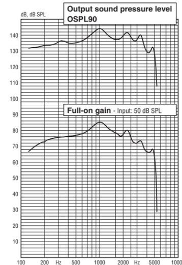
Frequency response with magnetic and acoustic input
