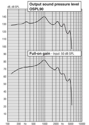
Frequency response with magnetic and acoustic input
