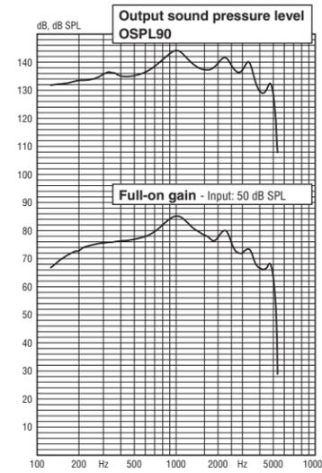
Frequency response with magnetic and acoustic input
