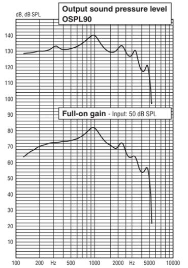
Frequency response with magnetic and acoustic input
