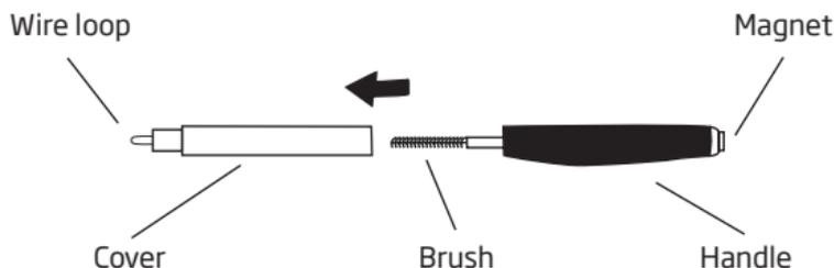
The MultiTool contains a brush and a wire loop for the special purpose of cleaning wax from the ear mold. Use the cloth to wipe clean the surface of the instrument.
