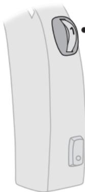
Use the volume wheel to mute the instrument by turning below setting 1 until it clicks. To reactivate the instrument, turn up on the volume wheel.
