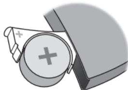
Insert the new battery into the battery drawer. Make sure the + side faces up.
