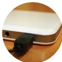
**STEP 2:** Plug the power cord into the power adaptor marked A.
