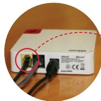
**STEP 4:** Plug the Tele Cord into the Phone Adaptor marked PHONE (yellow socket).
