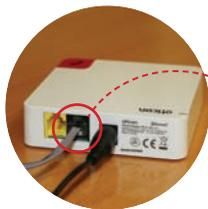
**STEP 2:** Plug the phone line into Phone adaptor marked LINE (black socket).
