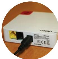
**STEP 2:** Plug the power cord into the power adaptor as shown.
