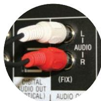
**STEP 2:** Plug the TV cord into the output jacks as shown.
