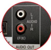
**STEP 1:** Locate audio output jacks on back of TV (typically labelled Audio Out).
