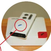
**STEP 1:** Place Streamer close to adaptor. Press pairing button until blue light flashes rapidly.
