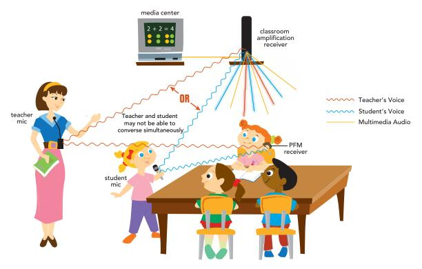
Microphone-Restricted Integration allows the teacher to transmit his/her voice directly to the student with hearing loss **and** the classroom amplification receiver. However, it does not allow the student to hear multimedia audio.
