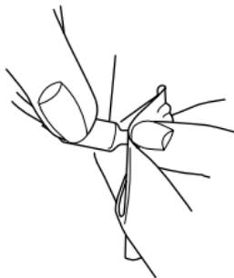
Under the dome you will notice a white wax filter attached to the end of the speaker. This is a wax filter that will keep debris from damaging the speaker. If this filter becomes clogged, contact your Hearing Care Professional for service and replacement of the filter.
