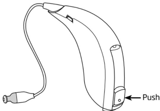
The push-button on your hearing instrument can be programmed to one of three functionalities.
