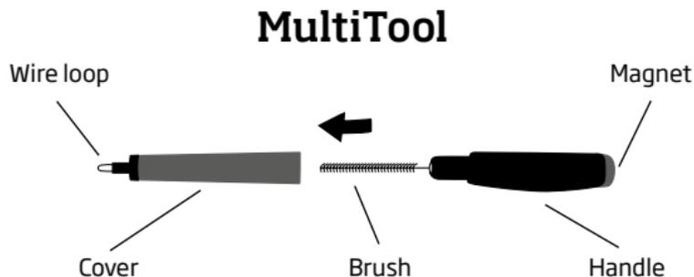
The MultiTool contains a brush and a wire loop for the special purpose of cleaning wax from the mold. Use the cloth to wipe clean the surface of the instrument.
