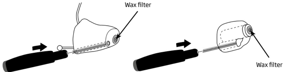
Replace the brush when necessary. Just pull it out of the tool and insert a new fresh brush. Press the new one firmly into the handle. Brushes can be purchased from your Hearing Care Professional.
