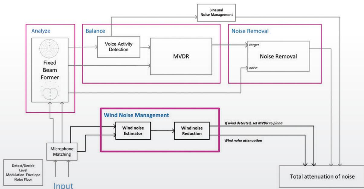
Figure 1: Wind Noise Management is, with OpenSound Navigator and Binaural Noise Management, part of the noise management feature on the Velox platform.
