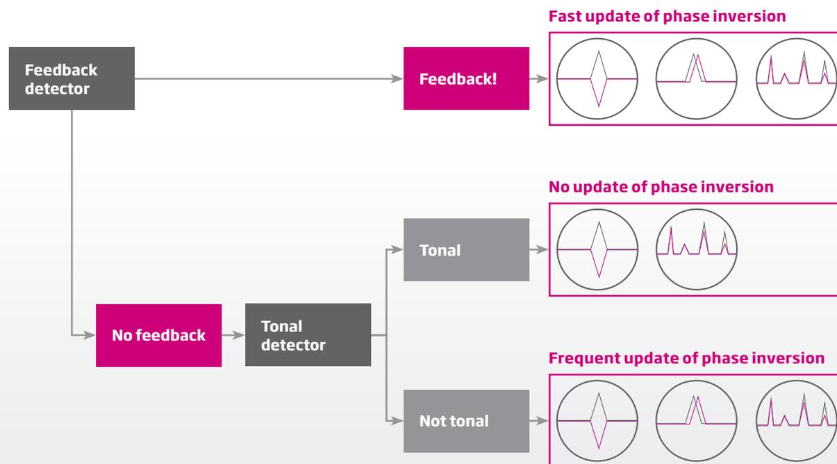
Figure 2. Schematic modes and detectors in feedback shield.
