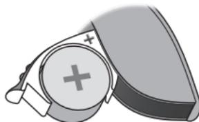
Insert the new battery into the battery drawer. Make sure the + side faces up.
