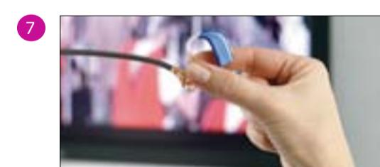
EN Hold the hearing aid near a television that is turned on. A buzzing sound will confirm that the telecoil is working.
