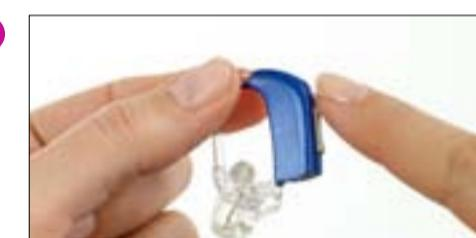
EN Checking the Telecoil (T-coil): A T-coil with a loop system broadcasts directly to the hearing aid when it is in the T-program. If your child uses a telecoil program you can also perform a listening check of this. Turn the hearing aid to the "MT" or "T" program.
