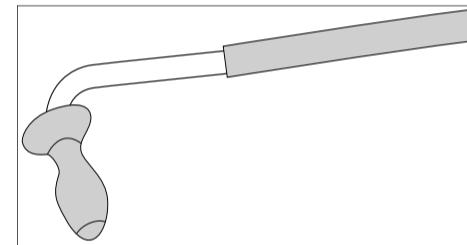
EN Undamped tube - for use with mild and moderate power hearing aids; NEVER use with Power instruments (risk of damage to normal hearing).
