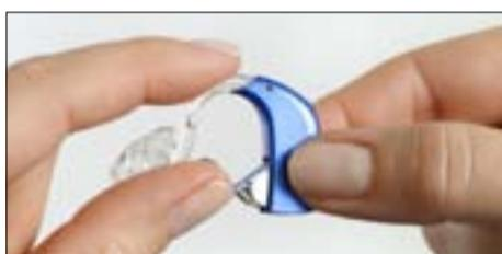
EN Turn the hearing aid off by opening the battery door.
