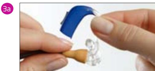
EN If you are checking a hearing aid that fits behind the ear, as shown, attach the other end of the listening tube to the earmould of the hearing aid.
