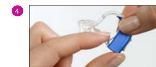
EN Turn the hearing aid on by closing the battery door. You should hear a start-up jingle, unless the jingle has been turned off by the hearing care professional.
