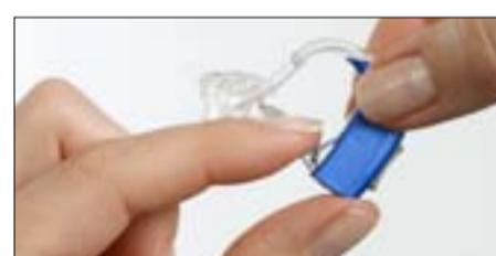
EN Turn the hearing aid on by closing the battery door. You should hear a start-up jingle, unless the jingle has been turned off by the hearing care professional.
