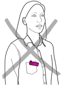
The microphone should point towards the speaker's mouth and be within a distance of 10 to 20 cm.
