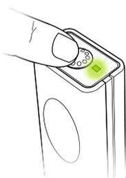
Tap the top of the microphone to check that the sound is heard in the hearing instruments
