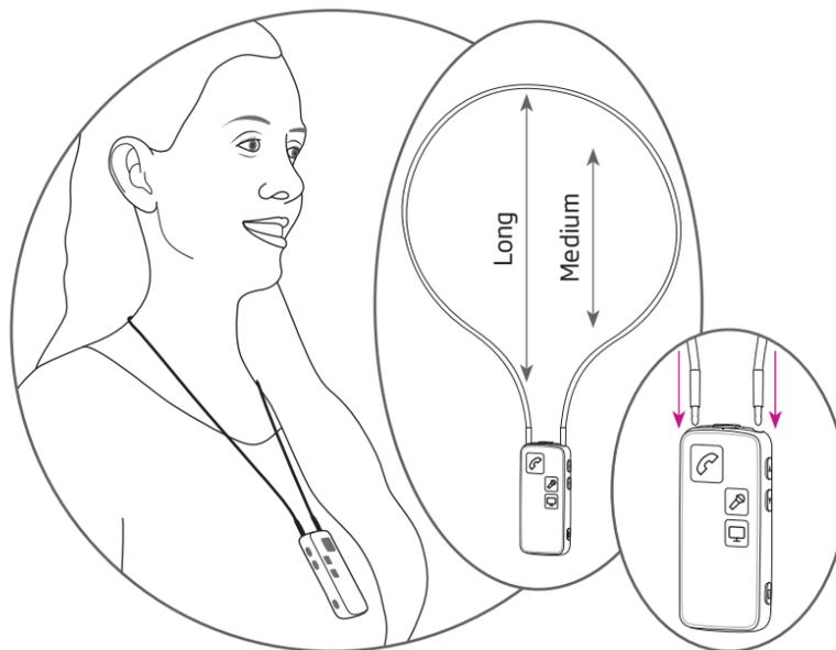
The neck loop is an integral part of the Streamer's electronic system. It is used as an antenna to transmit sound to your hearing instruments.
