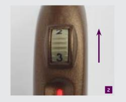
Insert a battery into Amigo Star, close the battery door, and roll the volume control past position 1.
